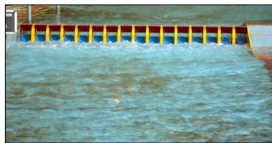
Performance of Stilling Basin for Gated Operation of Spillway, Q=18098.25 m<sup>3</sup>/s (75%) at MWL El. 240.561 m
