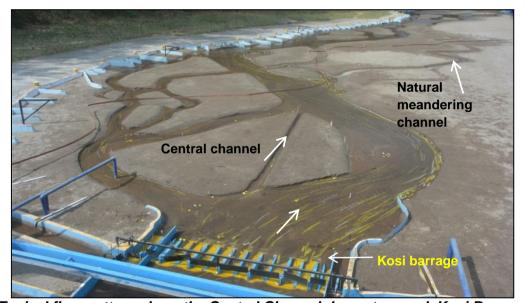
Typical flow pattern along the Central Channel downstream ok Kosi Barrage
