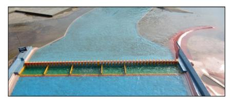
Flow conditions upstream of spillway for Q= 106187 m<sup>3</sup>/s and ungated operation of spillway
