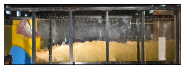
Flow conditions for gated operation of spillway Q=109000 m<sup>3</sup>/s at FRL El. 45.72 m and TWL El. 31.77 m
