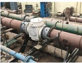
Micro hydro turbine unit fitted along the test line
