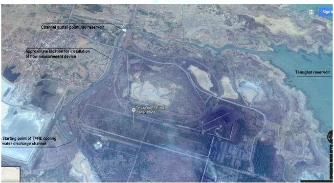
Location of flow measurement with respect to TVNL plant and Tenughat reservoir
