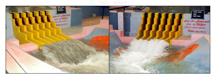
Flow condition for ungated operation of spillway, Q=13000m<sup>3</sup>/s (100%) at RWL EI 744.8 m
