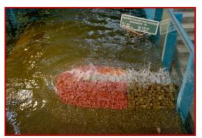
3-D Wave flume test for round-head portion
