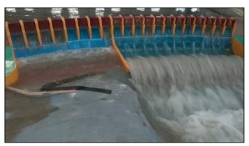
Flow conditions in the downstream with ungated operation of main spillway and gated auxiliary spillway at FRL El. 262.13 m
